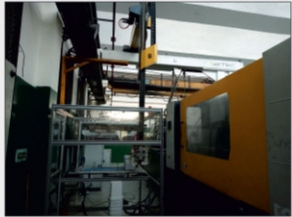
450 Tons Injection Moulding Machine with use of Robotics
