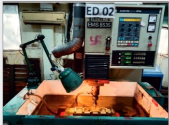
Electro Discharge Machining (EDM) Facilities
