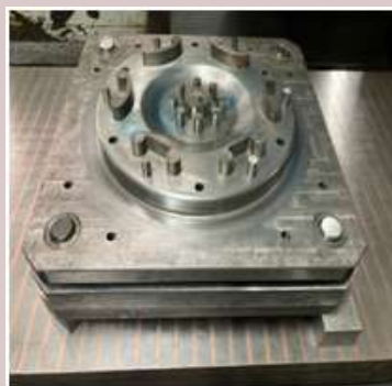
Automobile Industries Compound Die for Flex Plate (Alternate for Fly Wheel)
