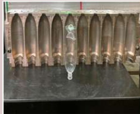
10 cavity Eye Drop bottle blow mould
