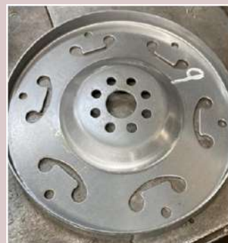
Automobile Industries Compound Die for Flex Plate (Alternate for Fly Wheel)
